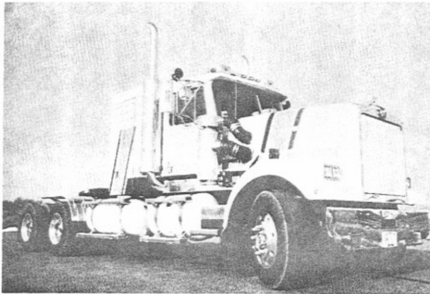
Figure 5.3/ Western Star Class Eight Tractor Equipped with a Cummins Engine Powered by Propane
