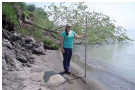
Emily Armstrong and Brent Zimmer surveyed to determine the 80th percentile for work along the Lake Erie shoreline. The 80th percentile means erosion control structures can be placed on the beach adjacent to the shoreline at the toe of the bluff, so long as 80% of the time the structures are high and dry for the effects of normal wave uprush from the lake, with the potential to be wet 20% of the time during storm events.
