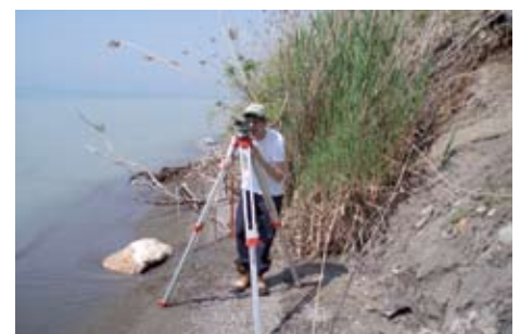
Emily Armstrong and Brent Zimmer surveyed to determine the 80th percentile for work along the Lake Erie shoreline. The 80th percentile means erosion control structures can be placed on the beach adjacent to the shoreline at the toe of the bluff, so long as 80% of the time the structures are high and dry for the effects of normal wave uprush from the lake, with the potential to be wet 20% of the time during storm events.
