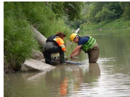
Staff prepare a PME miniDOT logger for sampling dissolved oxygen and temperature conditions in the Thames River.
