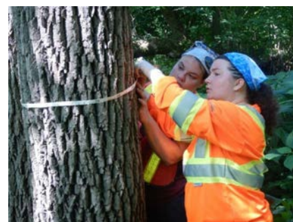
Staff taking the DBH (diameter at breast height) of an Eastern Cottonwood tree as part of ecological land classification (ELC) work at Big Bend Conservation Area.
